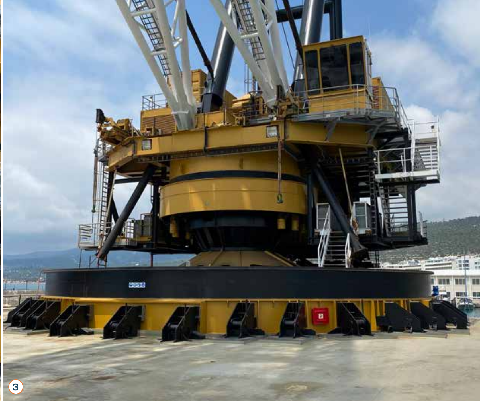
1 Sideview of the crane barge, with 180ton HD crawler crane | 2 1400ton main crane with sea-fastening for towage 3 1400ton main crane with sea-fastening for ocean towage
