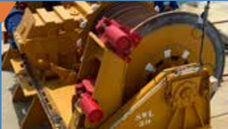
4 double drum 50 mT-rated pull winches
